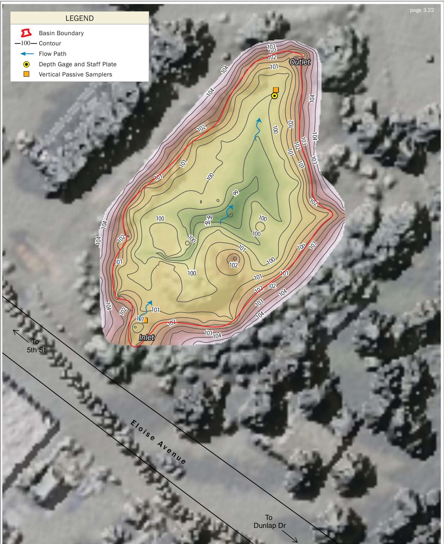
Figure 3.7D. Eloise Basin Site Map Shaded topographic contours of Eloise Basin. Elevations values are in feet, with a contour interval of 0.5 feet. Elevation is relative to Oft on staff plate where: Oft staff = 100 ft elevation
