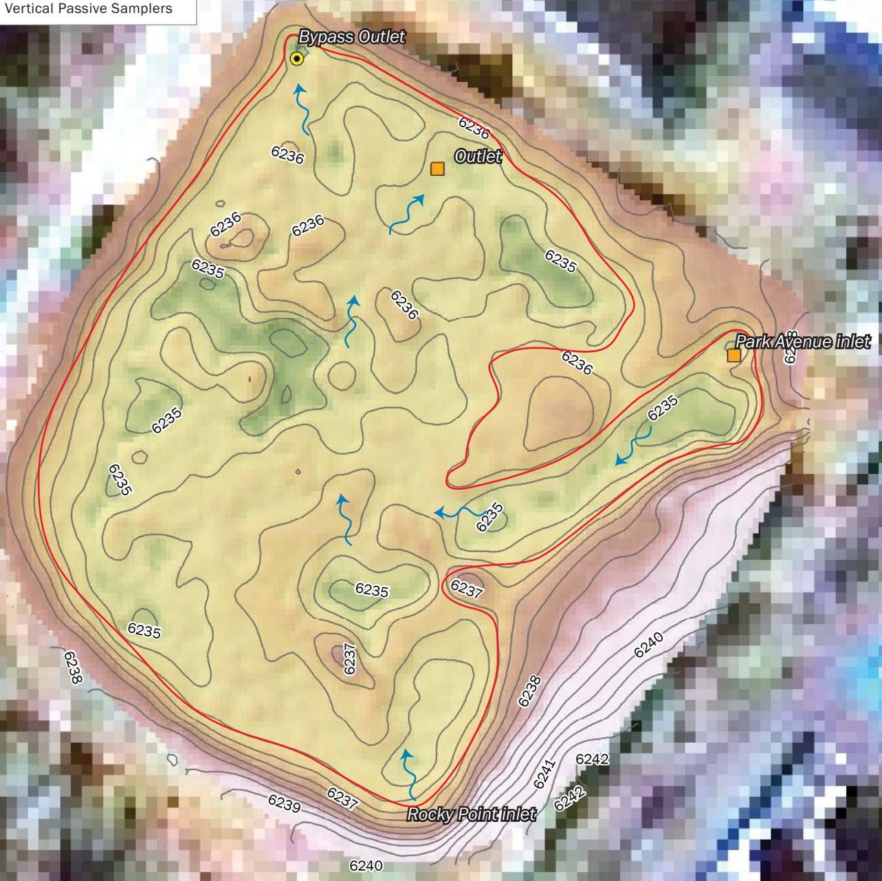
Figure 3.7B. PA1 Basin Site Map Shaded topographic contours of Upper Park Basin (PA1). Elevations values are in feet, with a contour interval of 0.5 feet. Elevation is relative to 0ft on staff plate where: 0ft staff = 6234.5 ft elevation
