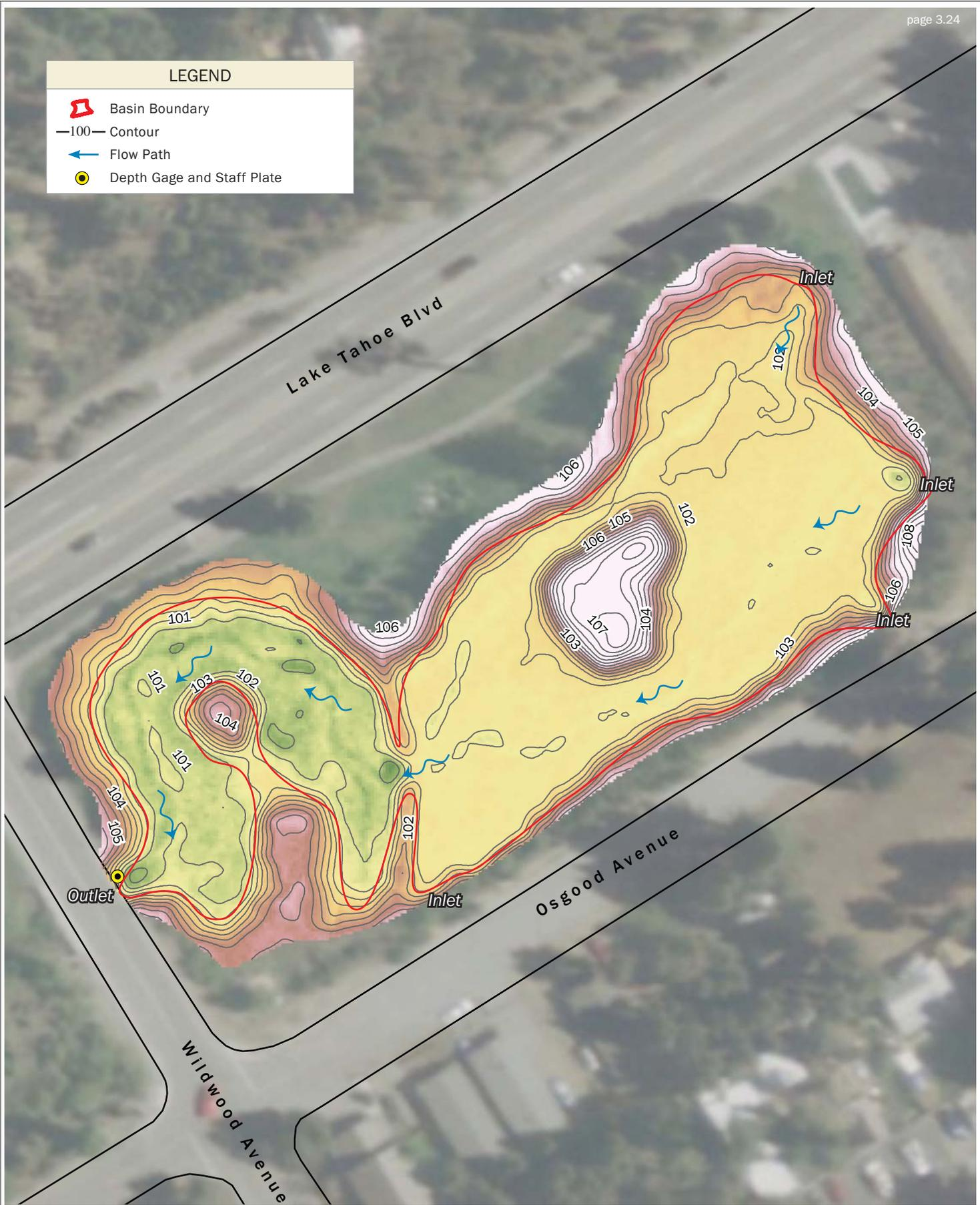
Figure 3.7F. Wildwood Basin Site Map Shaded topographic contours of Wildwood Basin. Elevations values are in feet, with a contour interval of 0.5 feet. Elevation is relative to 0ft on staff plate where: 0ft staff = 100 ft elevation
