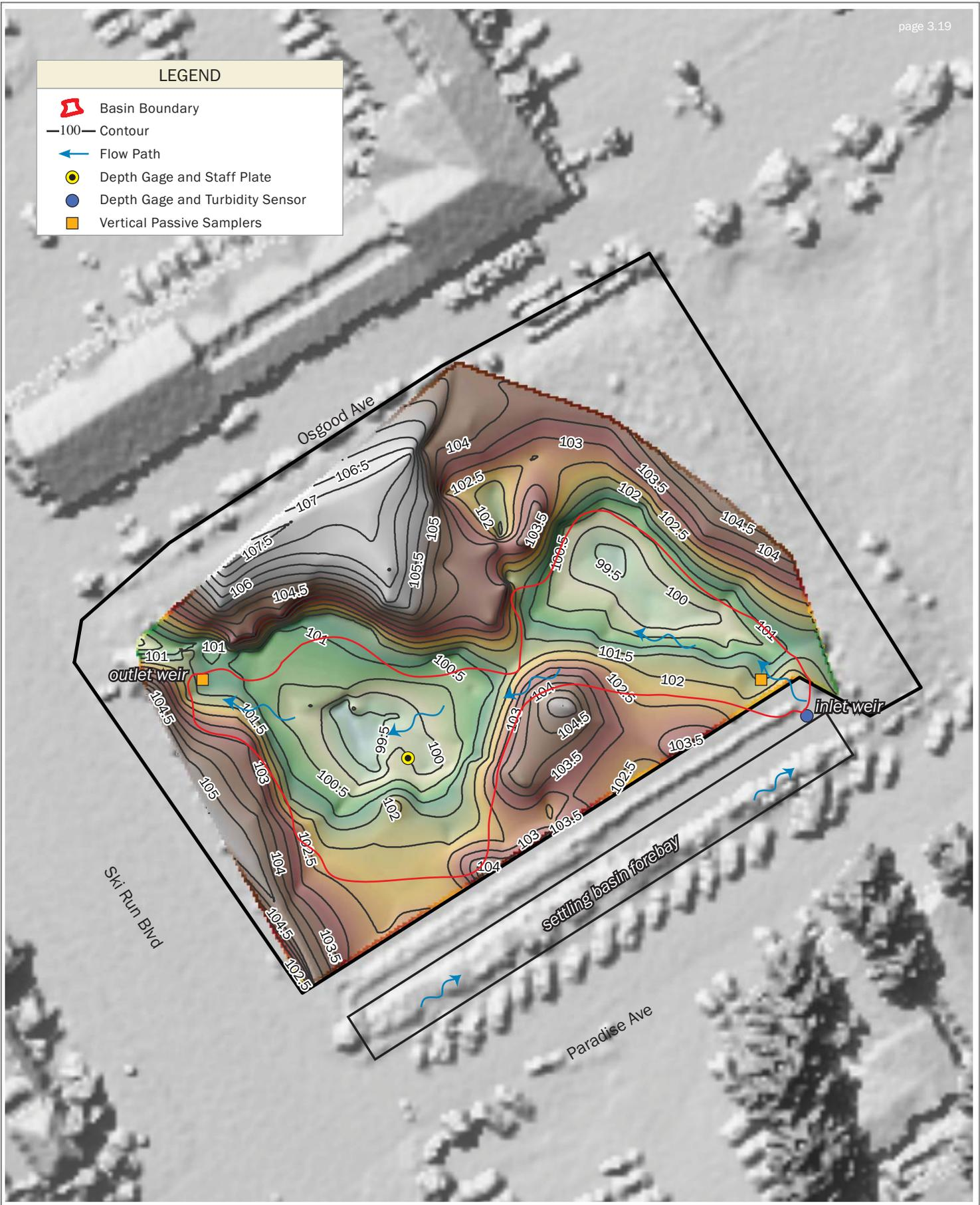
Figure 3.7A. Osgood Basin Site Map Shaded topographic contours of Osgood Basin plotted over a 2010 LiDAR data. Elevations values are in feet, with a contour interval of 0.5 feet. Elevation is relative to Oft on staff plate where: Oft staff = 100ft elevation
