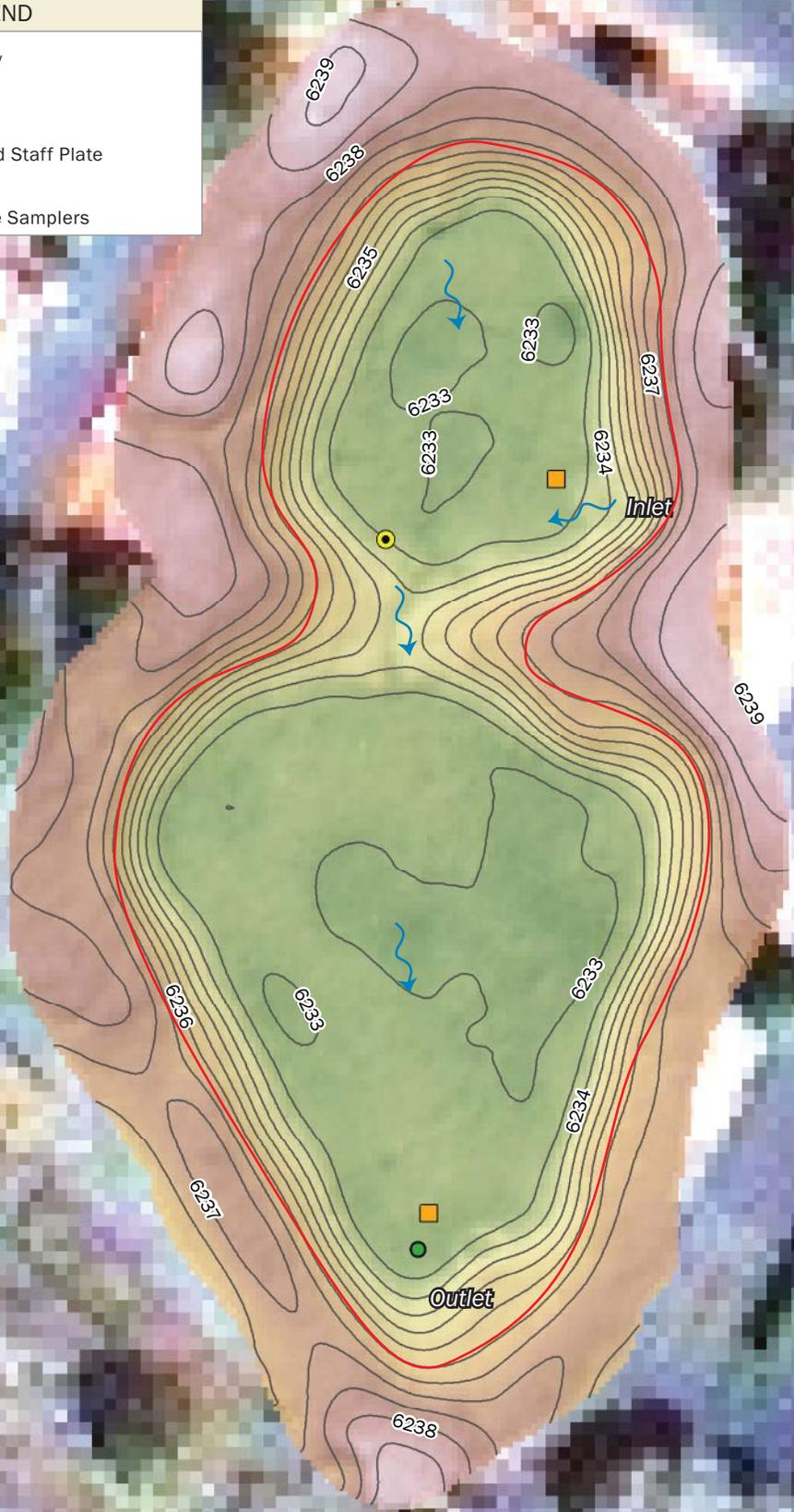
Figure 3.7C. PA2 Basin Site Map Shaded topographic contours of Lower Park Basin (PA2). Elevations values are in feet, with a contour interval of 0.5 feet. Elevation is relative to 0ft on staff plate where: 0ft staff = 6232.9 ft elevation
