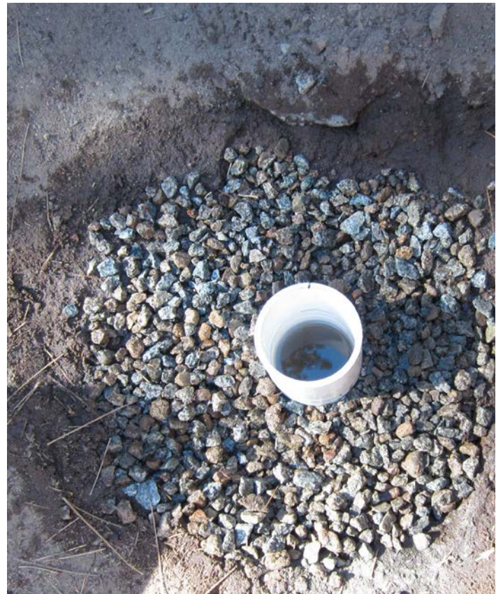
Top image shows configuration dimensions for In Situ experiments for both King's Beach soil series and beach sand. Bottom images show construction of an In Situ BMP in King's Beach soil with plexiglass cube to ensure uniform sizing (left image) and the planview of the constructed In Situ BMP (right image).
