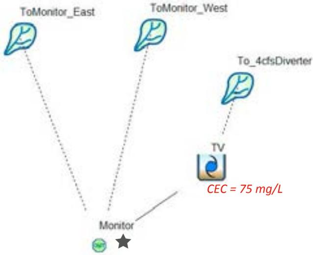
Simulation results are summarized at catchment outfall, which is representative of the monitoring location (★). Treatment vault modeled with CEC = 75 mg/L.
