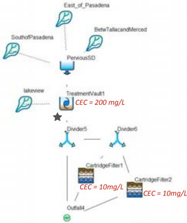
Simulation results are summarized below treatment vault (TV), but above cartridge filters (CF). Designated with ★ in schematic at left. Treatment vault modeled with CEC = 200 mg/L. This model assumes a significant portion of stormwater was bypassing the cartridge filters.
