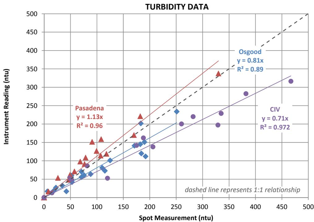
Depth spot measurements read from staff plates mounted on flume and/or weir next to instrument location (see photo in Chapter 3.2.4 of Osgood weir). Turbidity spot measurement taken of water flowing through monitoring location using Hach 2100P turbidimeter.
