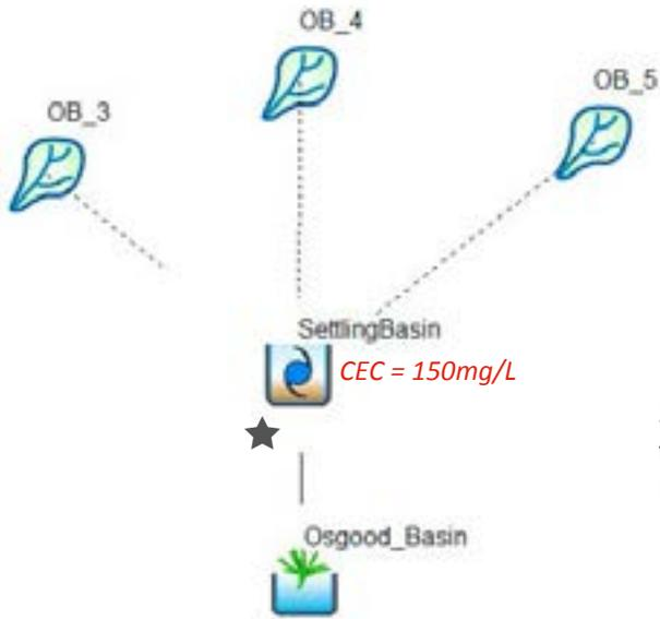
Simulation results are summarized below settling basin prior to wet basin (★). Representative of catchment monitoring location. Settling basin modeled with CEC of 150 mg/L.
