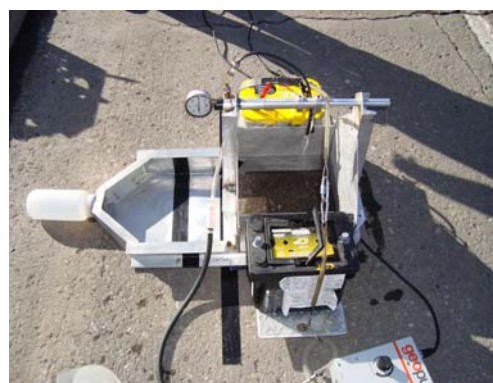
Portable simulator used to collect controlled road surface samples.
